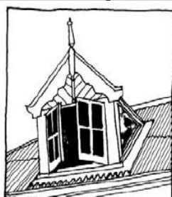
Dormer in a roof
